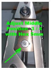
Adjust central position of the lever by setting the spring stop under the shift lever bracket with 5mm allenwrench. The shift lever (knob) should be in the neutral level 3./4.Gear about 5-8 deg. to the right >>>
