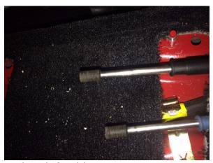
Remove the stock cable ends from the shiftcables
