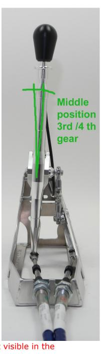
Adjust the Unibal-pushrod in the shifter by turning the rod until the pan of selection cable can pushed easily to the ball end of the Llever without offset. (almost shortest position)
