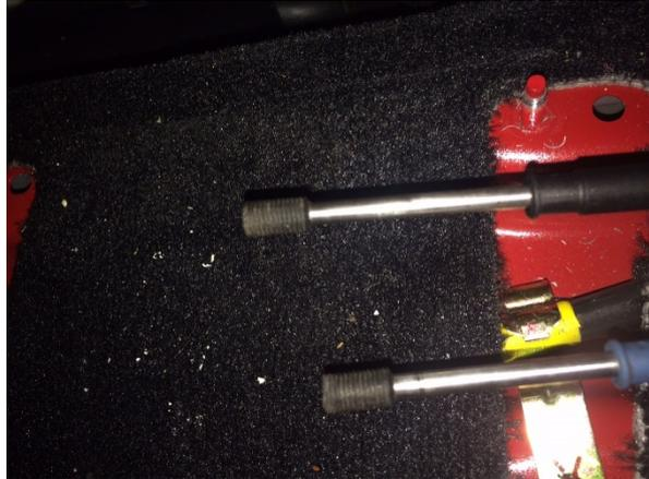
Remove the stock cable ends from the shiftcables
