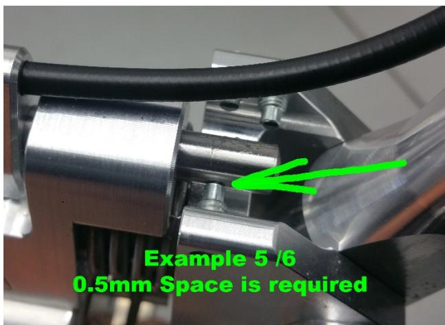
Check that all adjustment screws have about 0.5 mm play when gears are selected, not less and not more
