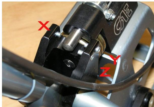
**CHECK:** If the lower part of the shift lever collide at the right side with the screw head of the pushrod you should adjust the central position of the shift lever slightly to the right, and start with step 1 "middle position"
