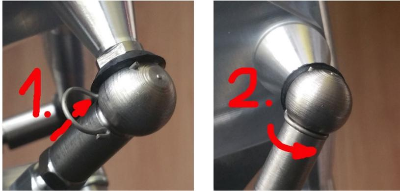
How to secure the ball pans by using the pin clamps
