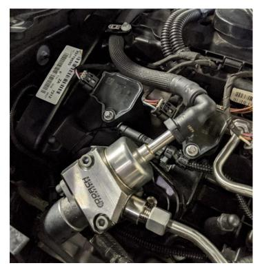
22. At this point double check all of your fuel connections, fastener torques, etc. and then reconnect the battery's ground terminal.
