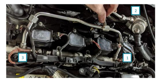
20. Lightly apply oil to the threads of the HPFP to prevent galling. If the nuts thread on effortlessly and bottom out with all the fittings well aligned, the three nuts can now be torqued.
