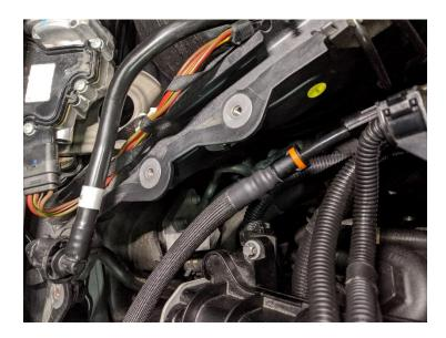
18. Using one of the spare E6 bolts removed in step 11, secure the low pressure line to the valve cover using the supplied bracket as pictured. Be sure to leave enough slack on the car's side to allow for engine movement.
