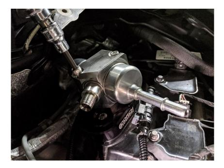
Pump to Flange Tightening Torque: 12nm
