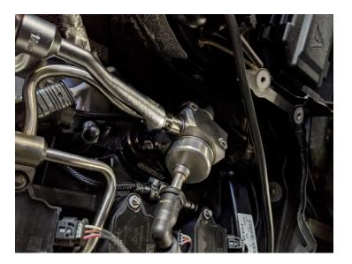
High Pressure Line Nut Tightening Torque: 31nm
