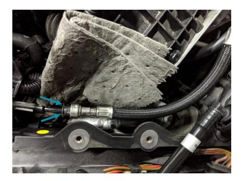
14. Lastly, remove the OEM high pressure pump using a T30 socket. Use **CAUTION** when removing the pump. The area must be VERY clean to avoid contaminating the pump and engine. You also must unthread each mounting bolt a little at a time to ensure the pump comes out STRAIGHT.
