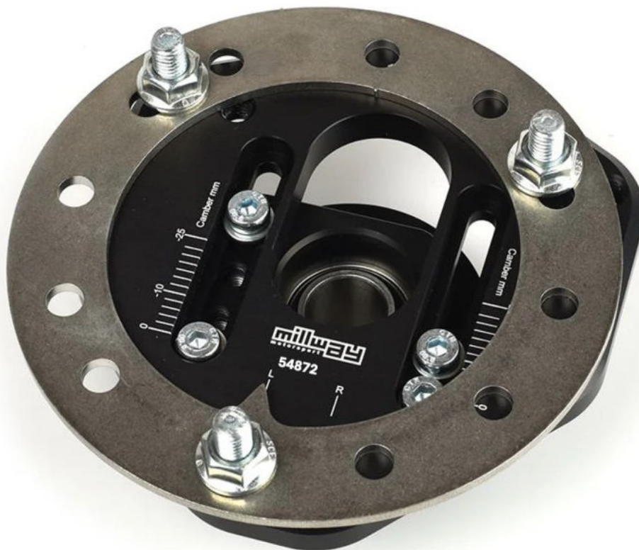
Adjustable strut bearings (Uniball): 54872
