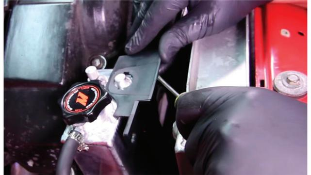
14. Reinstall the pop-clip that secures the top of the fan shroud. (1x pop-clip)
