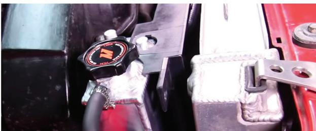
13. Attach the overflow hose to the port on the expansion tank, and then secure the hose with the worm-gear clamp. (1x worm-gear clamp)
