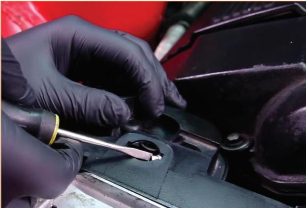
05. Disconnect the electrical harness from the coolant level sensor, located on the bottom of the expansion tank.
