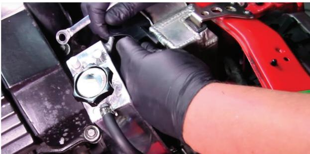
12. Slip the forward mounting peg on the top of the Mishimoto expansion tank into the hole where the bleeder screw seal was removed.
