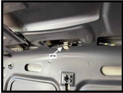
X710 On the tailgate Component plug (3-pin, black), license plate lights
