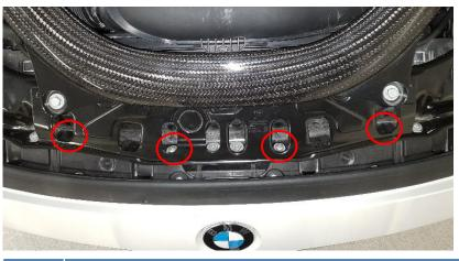
Where left and right air guids secures to the frame rails you need to remove these plastic clips, carefully push the air guide inwards while grabbing the clip and pry it out from its slot.
