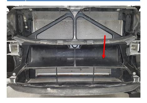
9. Remove 4x Torx T30 to release the upper plastic air guide.
