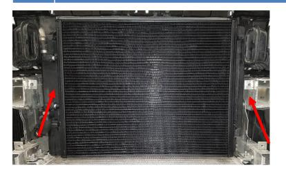
Drill a 5mm hole in the plastic tab that holds the radiator thru the do88 radiator bracket.
