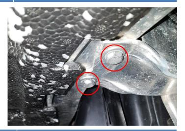
7. Loosen 4x Torx T45 that holds the crossmember and 2x T40 on top of it.
