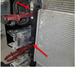
To remove the radiator, you'll have to push the radiator from the right side to the left side, carefully pry the plastic tab on the down right corner the opposite direction.
