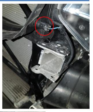
Use two hose pincher pliers to keep most of the **15.** coolant from draining out. Use a small flat head screwdriver and release the clips on the connectors, remove connectors from radiator and plug the connections on the radiator with the included 21mm silicone caps.
