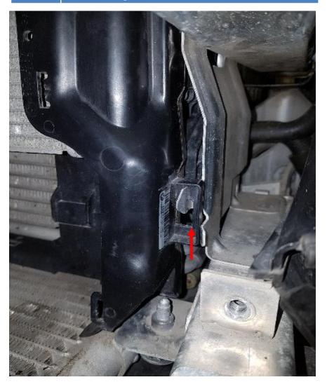
Use a small flathead screwdriver and remove the 13. plastic cover and use your fingers or a plier to push the two tabs together and use another plier to lift the plastic tab upwards, do this on both sides of car. Now you can carefully move the radiator assembly towards the engine to make more space
