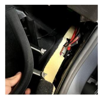
To thread the cable through later, we flip open the cover on the right side of the dashboard and expose the access into the dashboard.
