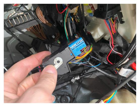
A yellow/white wire comes to pin 48 and a yellow/black wire comes to pin 47. If this is not the case, please send us a picture of your cable colors and the connector to coordinate the further procedure.
