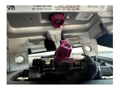
Remove the rear bezel of the screen with a plastic wedge. Start at the bottom and work
