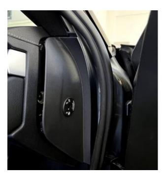
Now we lead a wire through from the side to the position of the speaker. Here you can shine through, have an orientation and see if the wire takes the right direction.
