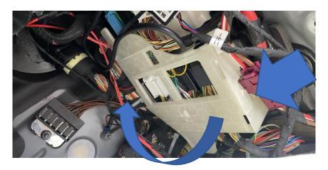
To release the connector, push in the latching lug and flip the lever. When the lever is turned, the connector is lifted out of the board. Now you can use a fine screwdriver to release the latch on both sides of the pin carriers and push the pin carriers out of the housing.
