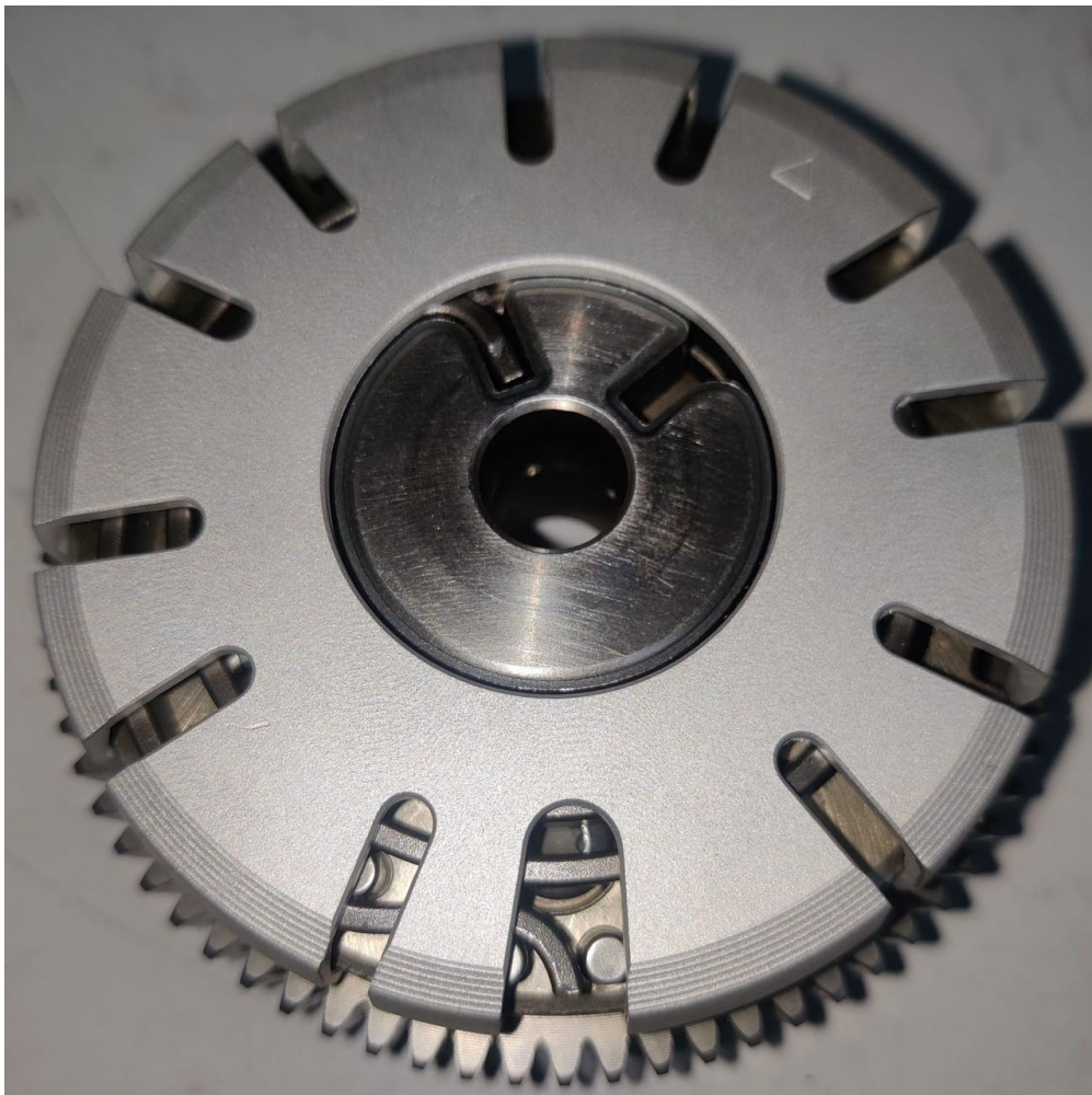
Figure 1: Ensure that the cover is pushed on straight from above without tilting so that all "wings" snap into place. Observe the positioning in the direction of rotation as shown in the following pictures.
