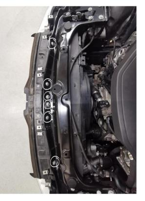
When the bumper cover is pulled out a bit you can reach the radar electrical connection and separate the wire from the bumper cover where the right break cooling duct is located.
