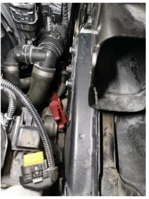
Remove the plastic lower radiator support by removing the 2 x T25 screws and releasing the clips from the radiator side supports.
