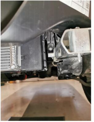
Now support the main radiator with a strap so you can remove the water-to-air intercooler radiator safely.
