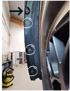
Remove the rubber sealing strip and remove the 6 x T30 and 2 x T20 screws marked in picture.
