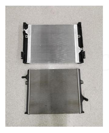
Transfer the radiator side supports to the do88 Performance radiator. To ease the bleeding process we recommend you pre-fill the radiator and block of the connections with the included silicone caps.
