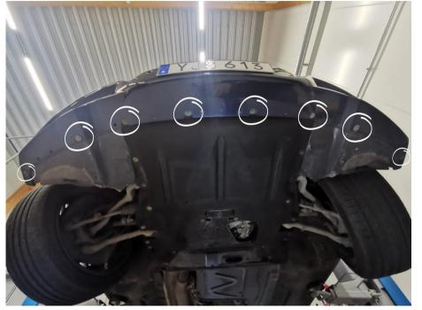
Remove the 8 x 8mm hex screws circled in the picture.
