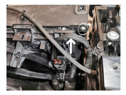
Remove the T25 screw holding the upper radiator support plastic on the left side .
