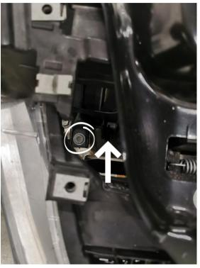
Remove the 2 x T40/13mm Hex screws and the T25 screw holding the headlight. Do the same on the right side. Remove the plastic lid and disconnect the radiator pack upper support pin on both sides.
