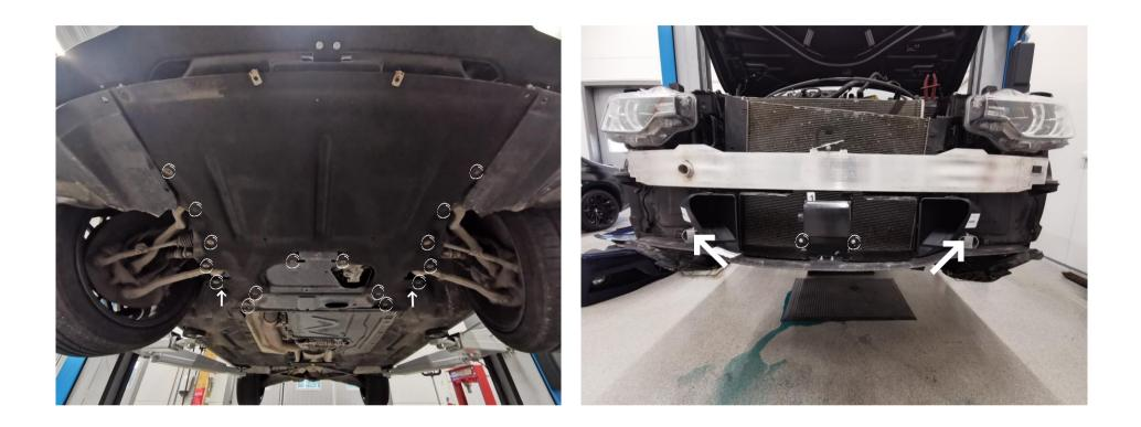
Now remove the 18 x 8mm hex screws that holds the underfloor and then remove underfloor.
