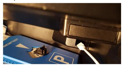
With LCI2 models, the small cover has been omitted, the USB cable can alternatively be routed through an opening under the rubber mat.
