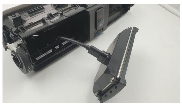
If the "retaining clip" is still on the left in the fresh air grill, remove it and attach it to the left side of the display. First insert the display on the hazard warning light side and then fold in the other side.
