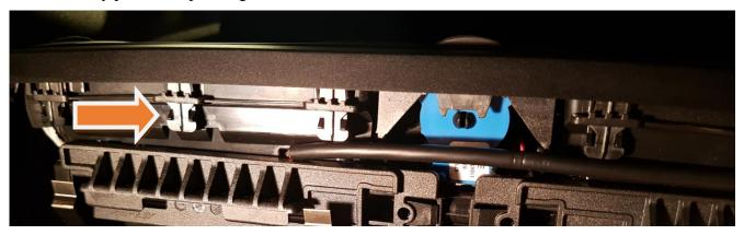
Route the display cable into the footwell on the passenger side.
