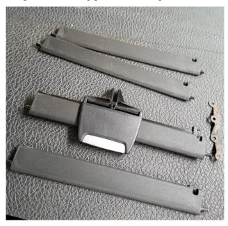
The second part of the grill can be easily removed by pulling apart the fresh air grill a bit:
