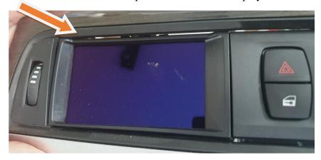
at the top, make sure that the retaining clip is correctly seated in the guide, then snap the panel into place.
