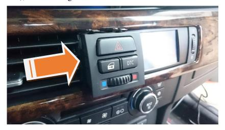
The fresh air vent is attached to the interior trim with two 8mm nuts and several clips. The two nuts are on the left and right sides.
