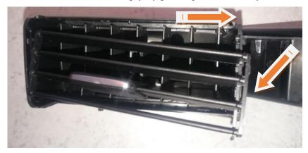
To remove the other part, the housing must be gently pushed apart.
