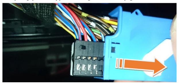
Now the cables Pin 1 (CAN\_High with the color red / blue) as well as Pin 2 (CAN\_Low with the color red) are pinned out. Use a small flat-head screwdriver, a needle or something similar. The crimp contacts have a flag which works like a barb. This flag must be pressed and at the same time carefully (!) Pulled on the cable.
