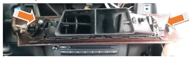
The clips must be unlocked carefully with a flat-head screwdriver.
