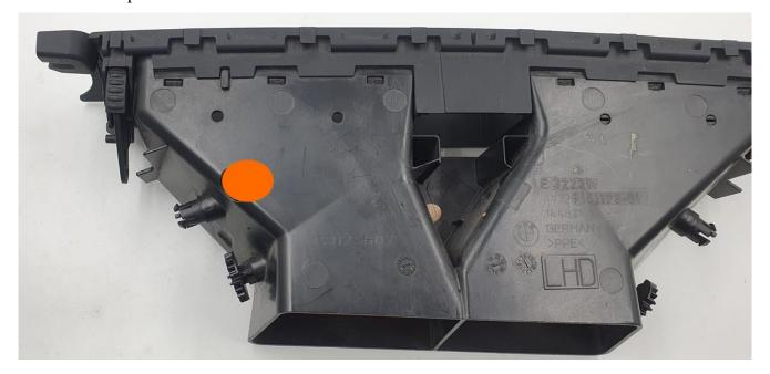
Deburr the hole a little so that no sharp edges damage the cable.
