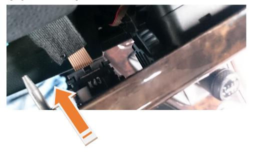
When the start / stop button is completed, the bar can be pulled out a little bit further.
