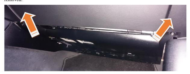
Now the cover can be carefully drained. Attention, there is still a plug connection of the footwell lamp to separate.
