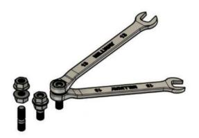
Two nuts on the longer threaded side of the stud bolt screwed together so that they no longer If the nuts
