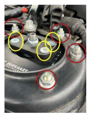
9. As marked in red in the adjacent figure, the spacers and nuts must now be mounted. The
