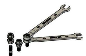
Two nuts on the longer threaded side of the stud bolt
