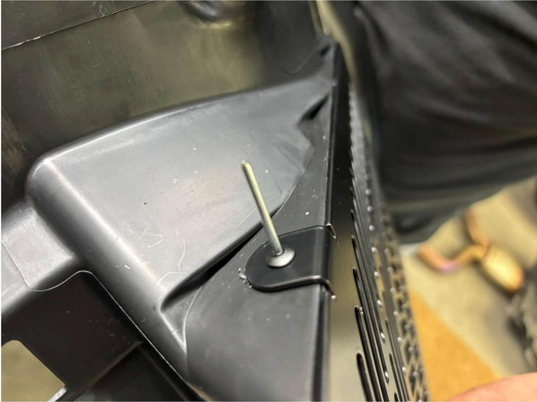
After drilling the hole in each upper tab, the rivet must be set as shown.
