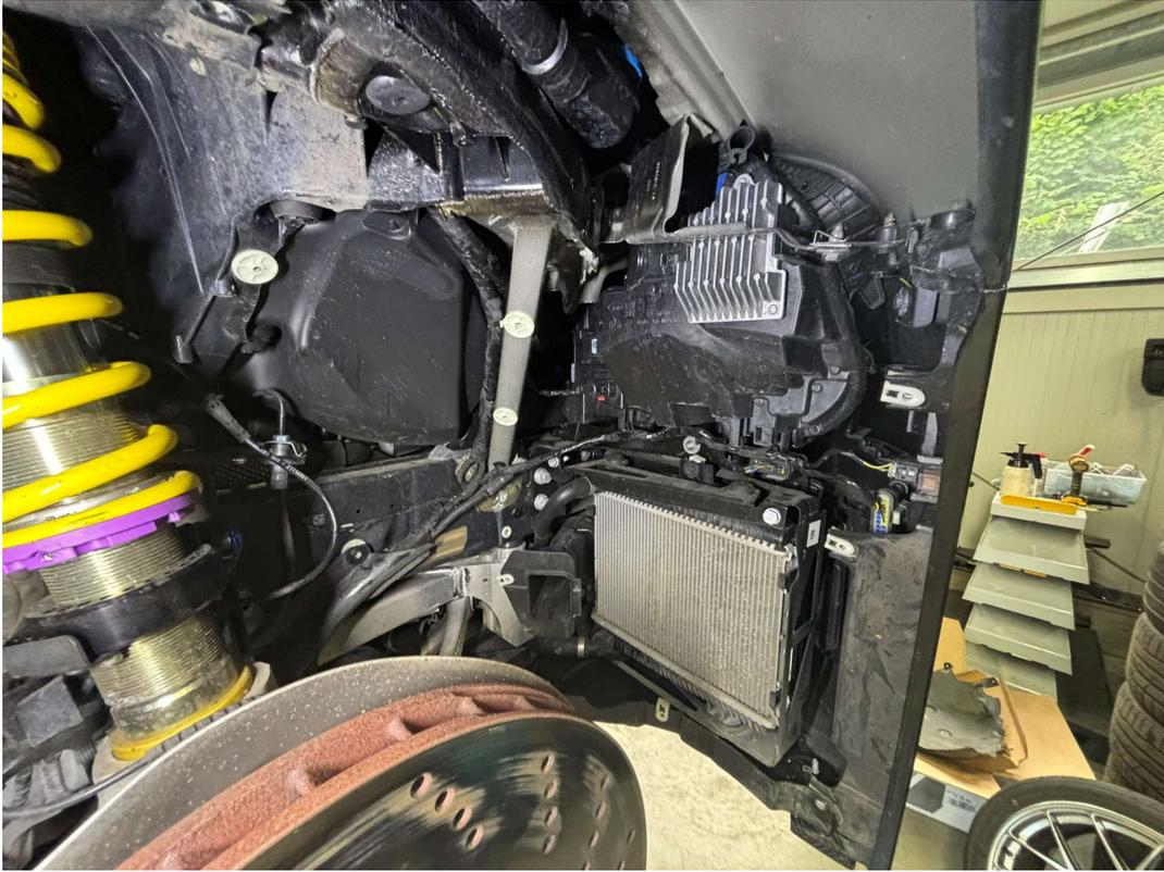
Carefully remove the front wheel arch liner, making sure that the plastic nuts are not displaced or damaged
