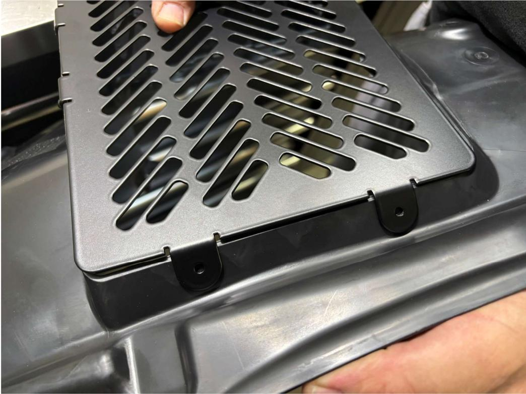
Now drill the holes for the two side tabs, keeping the grille securely in position.
