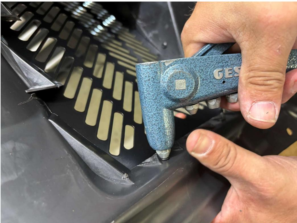
Now rivet the tabs of the previously drilled holes from the opposite side as shown here.
