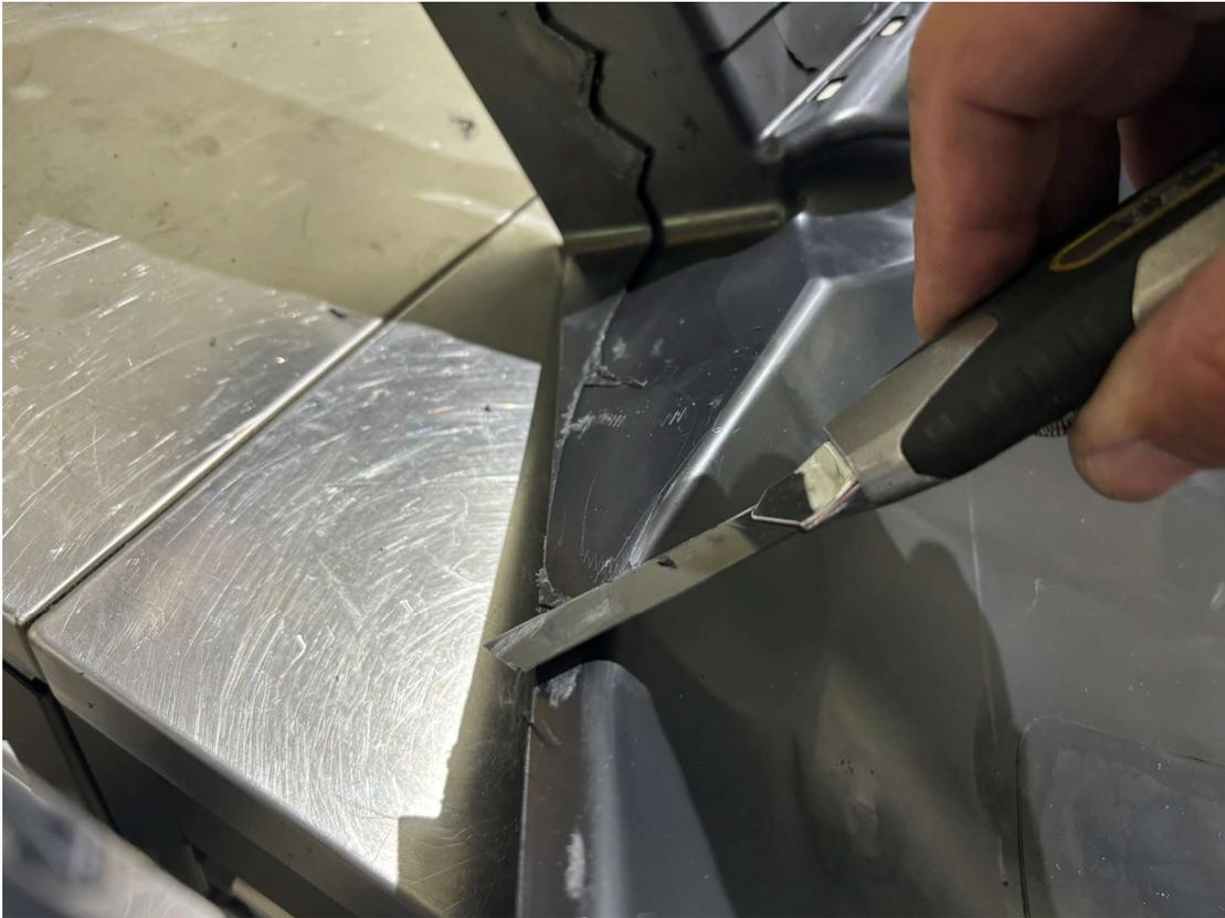
Protruding remnants can be carefully removed with a utility knife.
