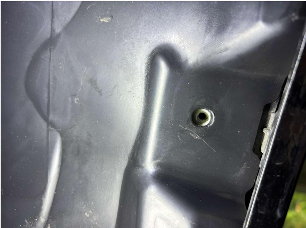
Position the wheel arch liner back into its designated place. Make sure all the holes align with the threaded inserts
