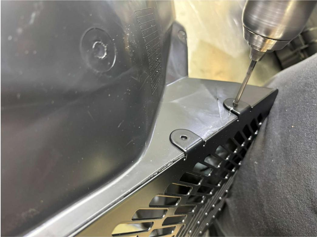
Drill holes for the top two tabs using the 4mm drill bit, keeping the grille securely in position.
