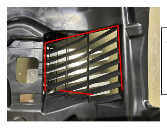
Carefully cut off the struts along the red line.
