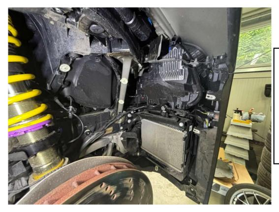
Carefully remove the front wheel arch liner, making sure that the plastic nuts are not displaced or damaged.
