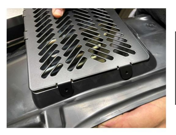
Now drill the holes for the two side tabs, keeping the grille securely in position.
