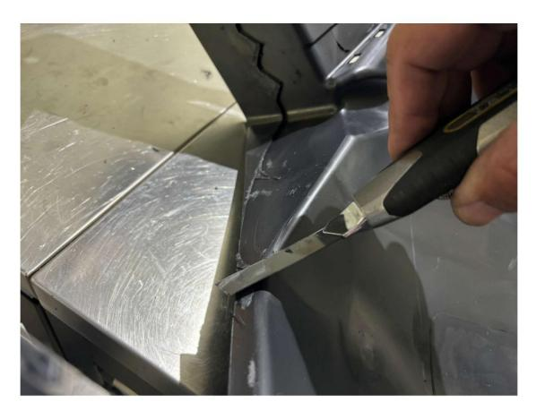
Protruding remnants can be carefully removed with a utility knife.
