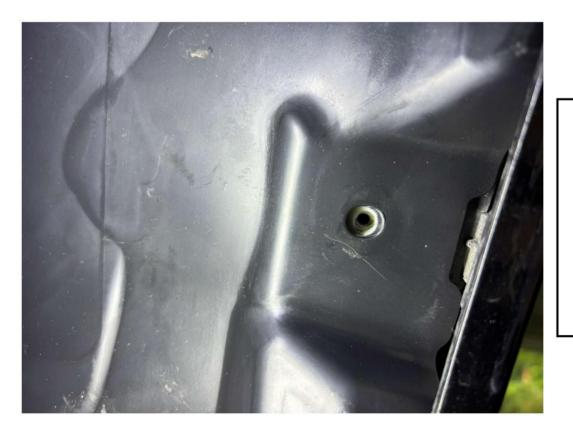
Position the wheel arch liner back into its designated place.
