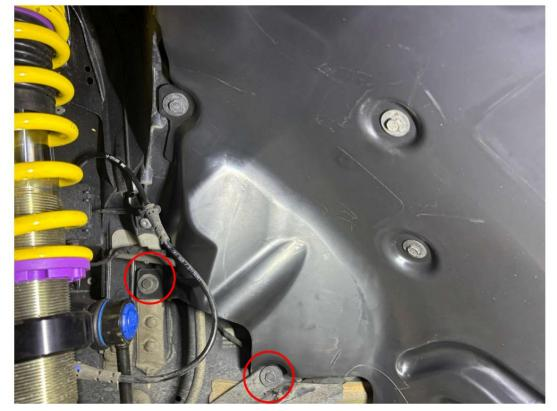
Remove the screws of the front wheel arch liner.
