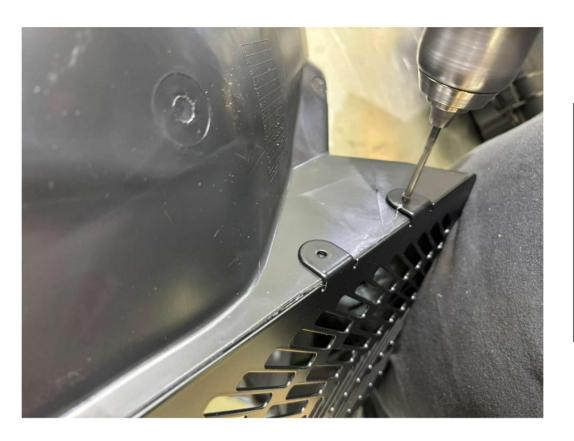
Drill holes for the top two tabs using the 4mm drill bit, keeping the grille securely in position.
