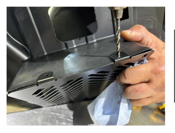
Now carefully drill the holes for the last two tabs.
