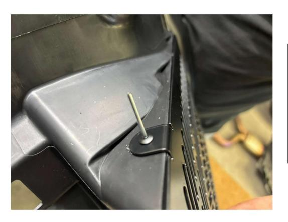
After drilling the hole for the single top tab, the rivet must be riveted as shown.
