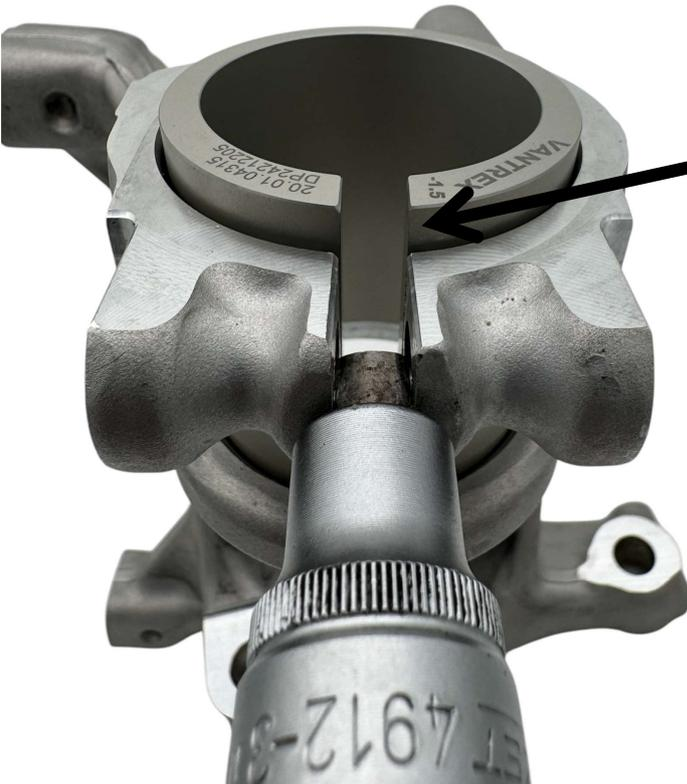
Then insert the Vantrax Camber sleeve so that the opening of the sleeve is flush with the opening of the steering knuckle.
