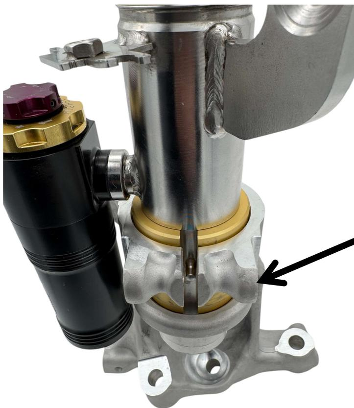
Remove the bolt at the rear of the steering knuckle. Then remove the bracket for the brake line.
