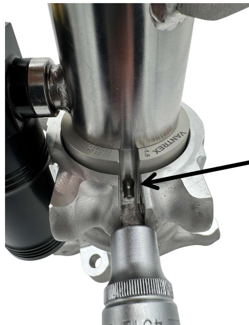
Use a transmission jack to push the steering knuckle into the stop when spread. Check that the sleeve and guide pin are still in the middle.
