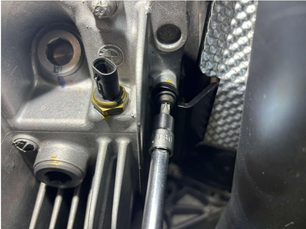
Fasten heat shield using supplied screws and one washer each.
