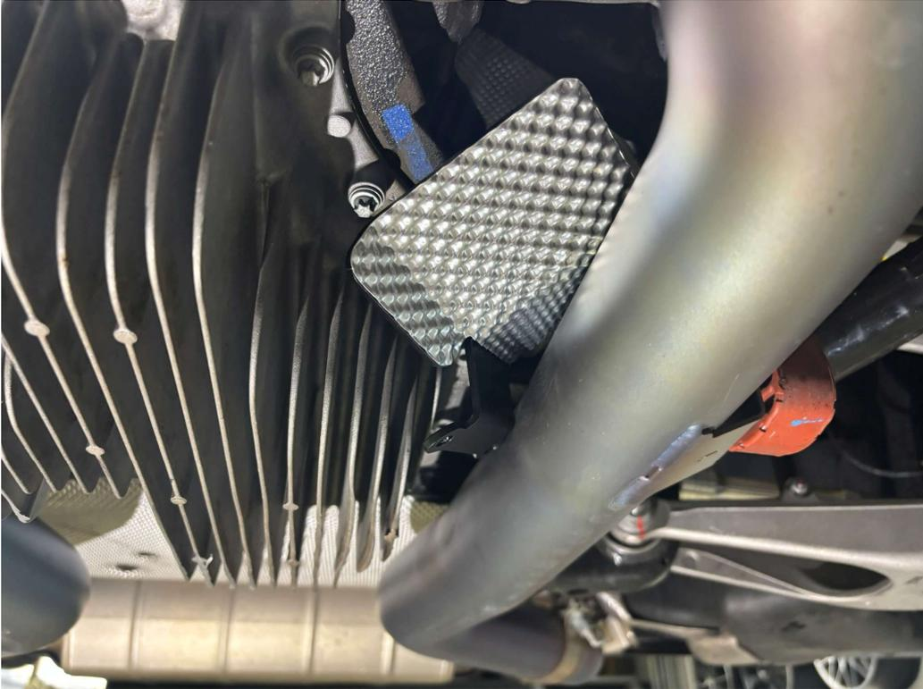
Insert heat shield on left side from front, centered between differential and exhaust system.
