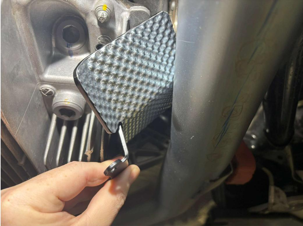
Insert heat shield on right side between differential and exhaust system, align correctly
