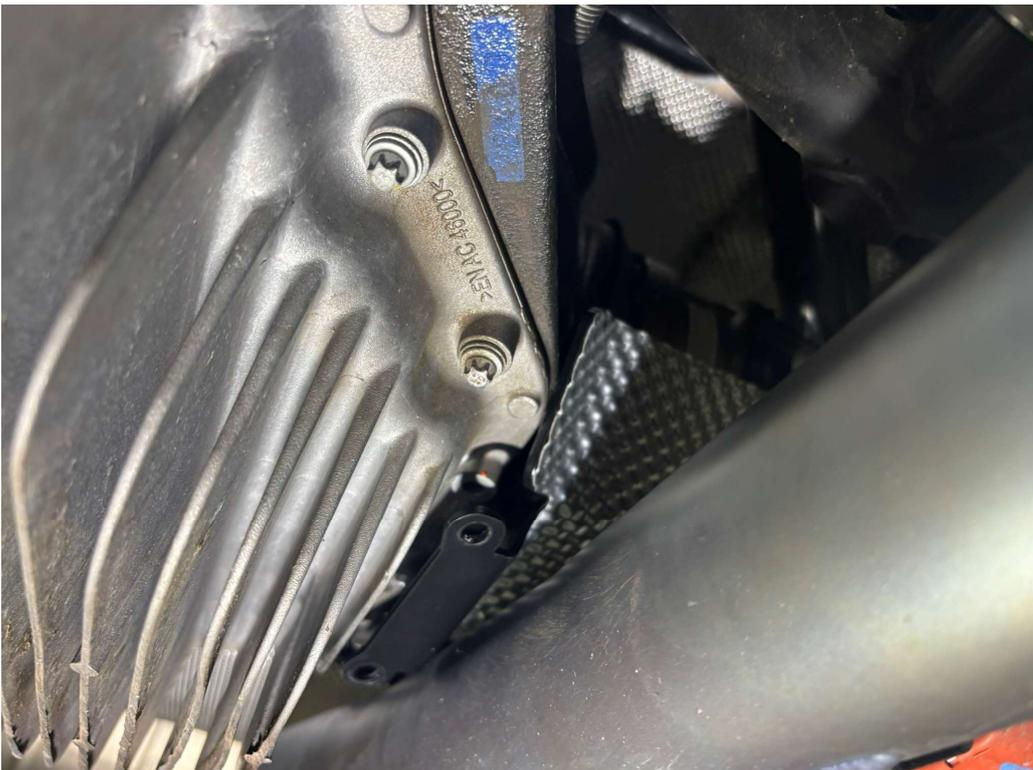
Fasten heat shield with supplied screws and one washer each, tighten to 12 Nm.
