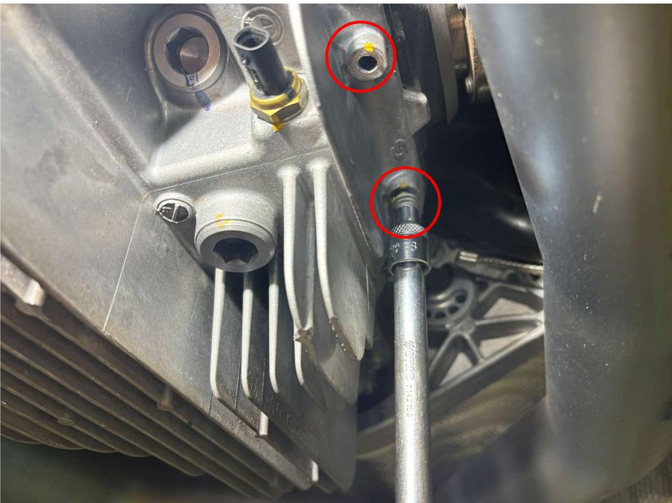
Remove the two oil pan bolts from the differential on both the left and right sides.
