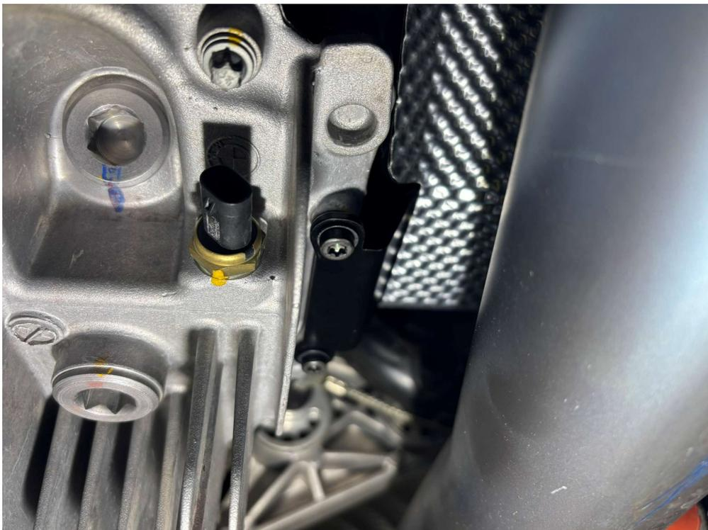
Tighten screws to 12 Nm using a torque wrench.
